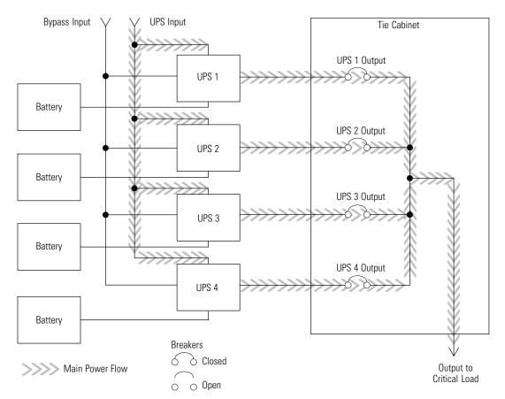
Figure 6-18. Path of Current through the UPSs in Normal Mode – Distributed Bypass
